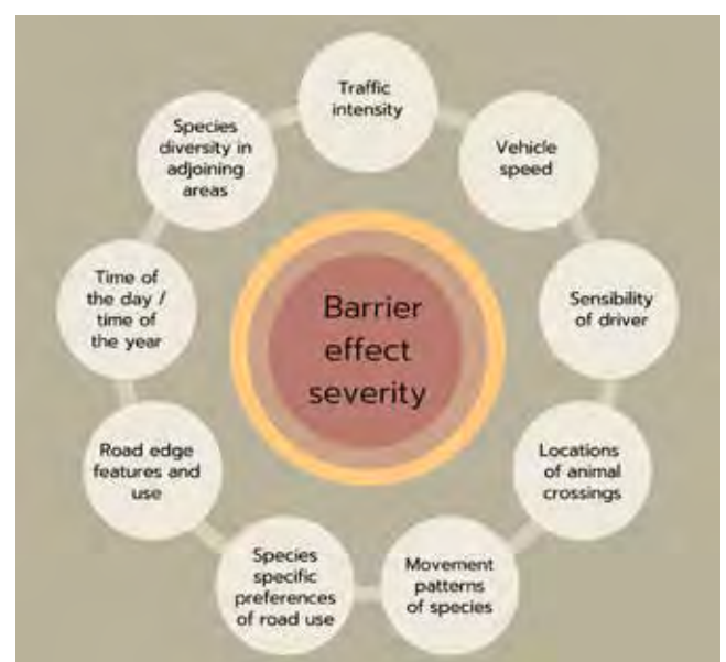
Figure 5: Factors influencing the severity of barrier effects on species and their free movement across LTI © Mary Collins / CLLC, adapted from Wildlife Institute of India
