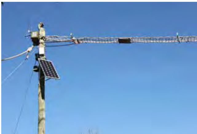
Wildlife cameras and passive integrated transponder (PIT) tags mounted at the end of a canopy bridge in Australia. PIT tag readers are technologies used to track the movement of individual animals that carry internal microchips. © Rodney van der Ree
