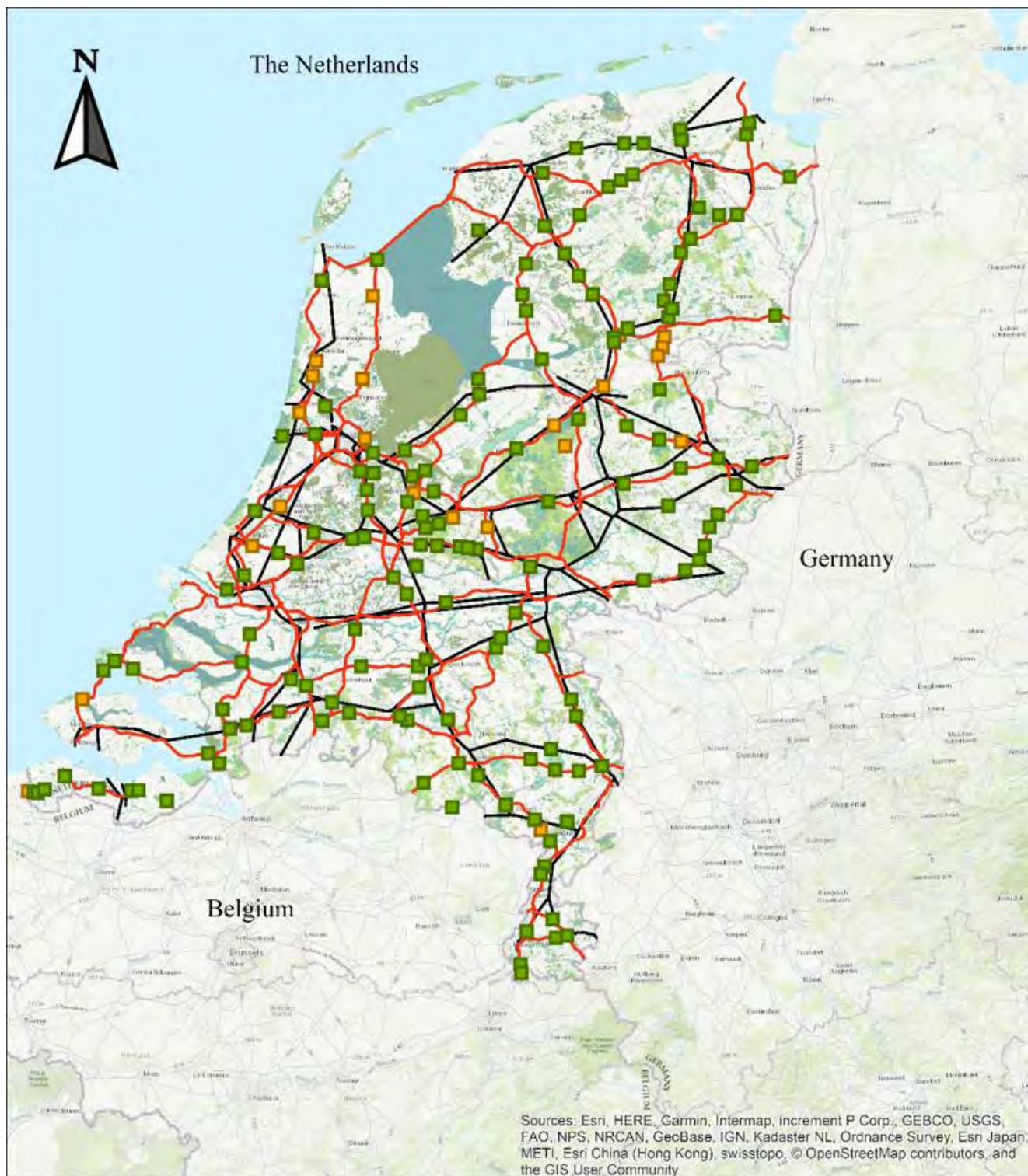
Figure 15: Locations of wildlife crossing structures (green) across Dutch national highways (red) and railroads (black); part of Netherlands' Multi-Year Programme for Defragmentation (MJPO). Concluded in 2018, the programme was able to mitigate approximately 60% of all the ecological barriers caused by the national infrastructure system, and as of 2017, there were almost 2,100 wildlife crossings for motorways and provincial roads. © Sijsma et al., 2020
