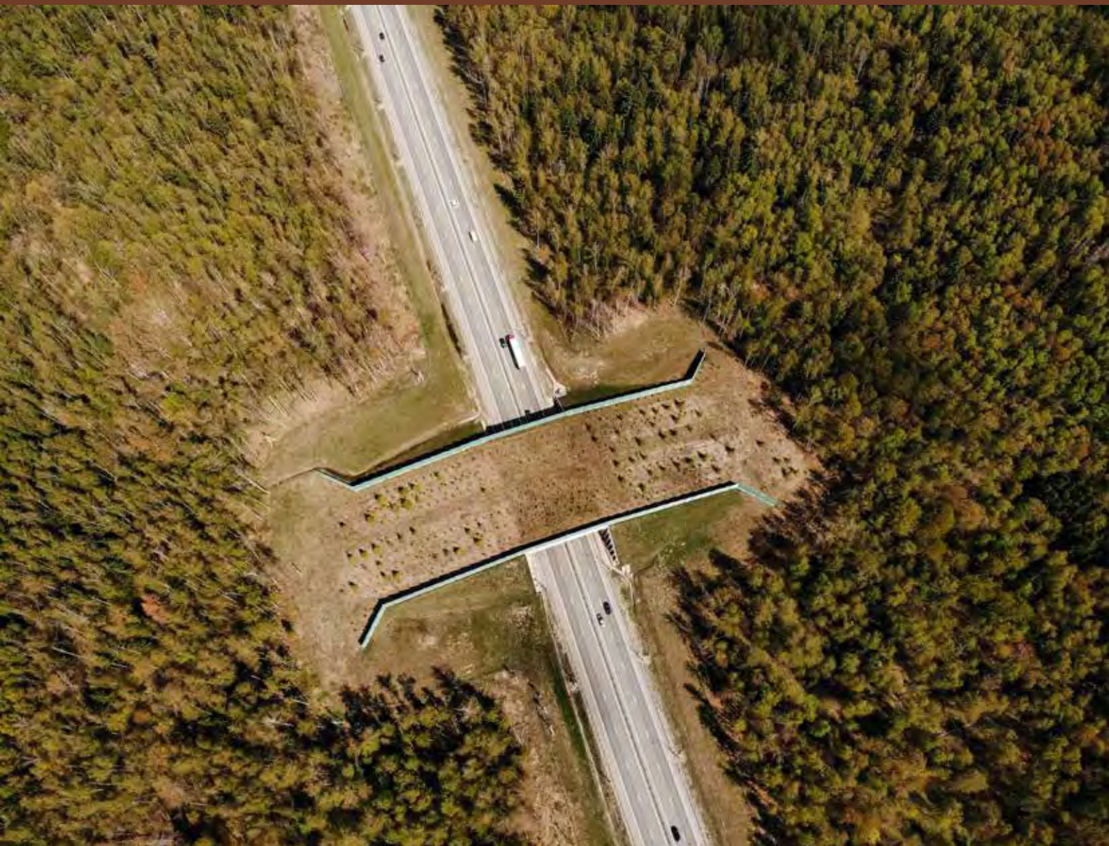
One of Russia's first wildlife overpasses, Route M3, Kaluga, Russia © Adobe Stock
